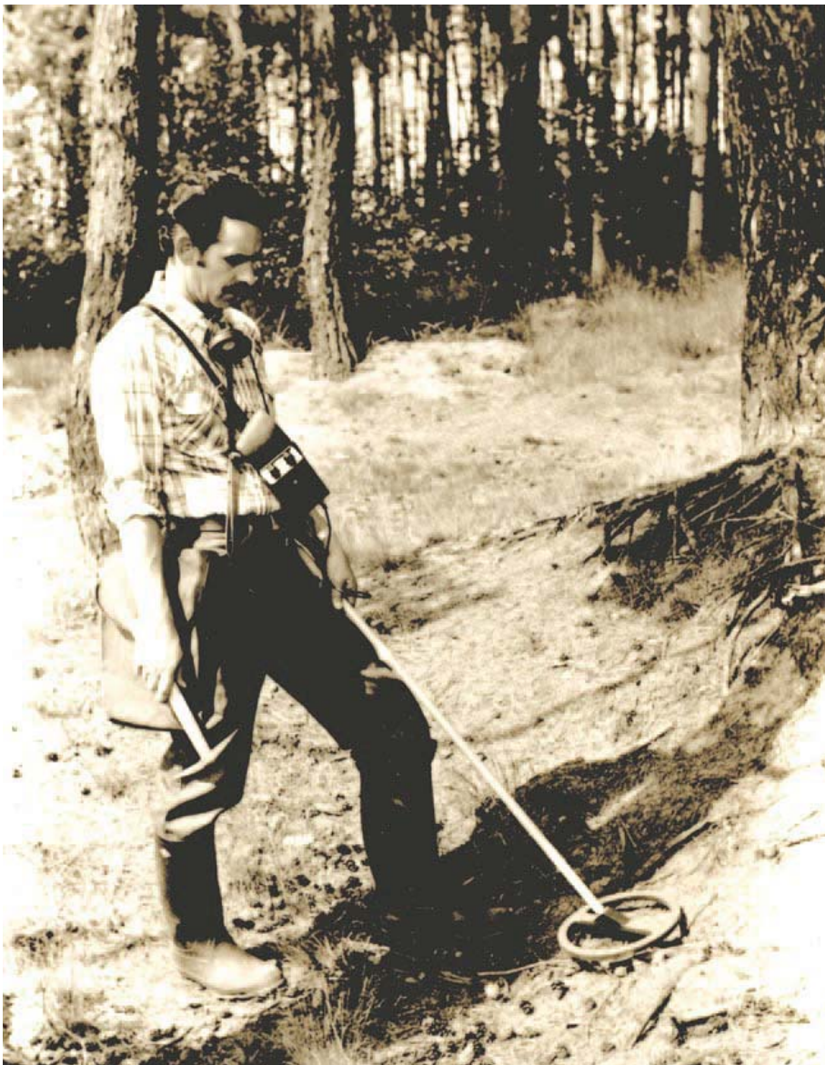
Fig. 11 Detector EB 710 (sine wave system in operation)
