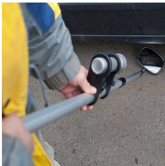
EFIS® 1 inspection mirror with torch
